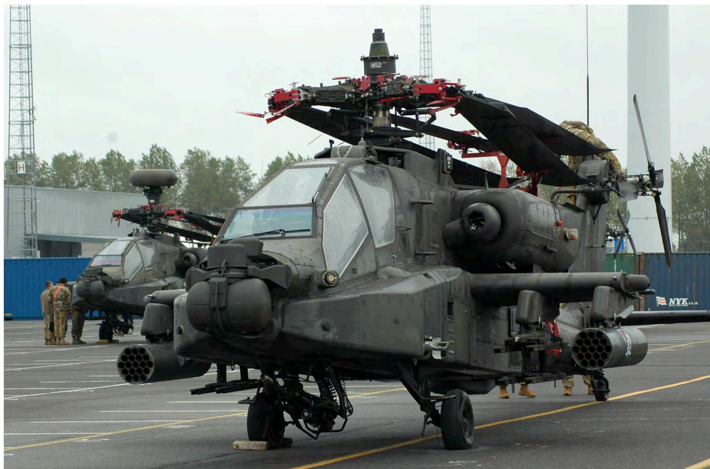
Two AH-64Ds from B/3-17 CAV (ARB) in the port of Zeebrugge. The one in the rear is equipped with the radarhead for the Longbow radar.
