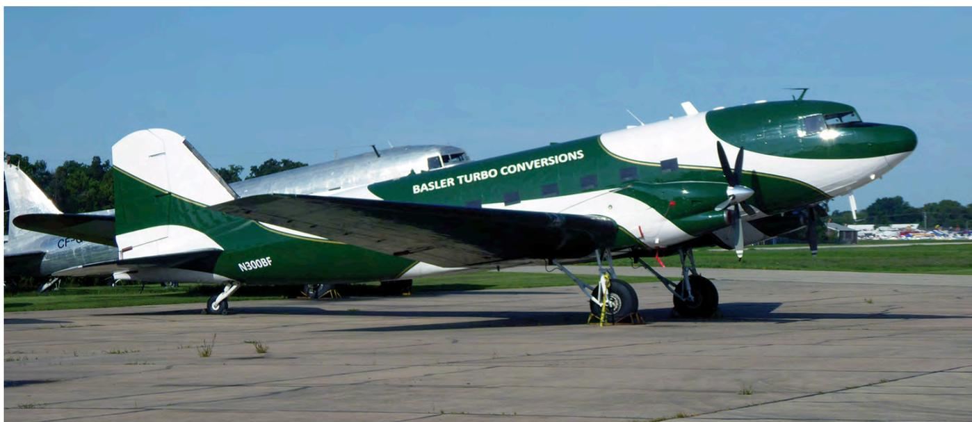
This 1943-built C-47 was delivered to the US Army as 43-49483 and transferred to the Royal Air Force as KK160. In 1987 it was bought by Basler which converted the aircraft in 1998 to a BT-67. Since 2017 it sports this new green/white livery. (Oshkosh (WI), 25 July 2018, Ad Jan Altevoigt)
