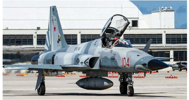
VFC-111 F-5N 761531 "AF-104" 2017 (3 tone gray scheme with lo-viz shark mouth and rudder markings). In order to be able to fly for a longer period of time, all the F-5s carry an external centreline fuel tank. The downside is that this tank degrades the performance of the aircraft in terms of G- forces. (George Karavantos)
