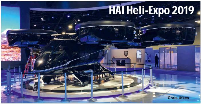
The 'nexus of transport and technology and of comfort and convenience' according to Bell. The hybrid-electric vertical takeoff and landing (eVTOL) aircraft was one of the highlights at this years Heli-Expo in Atlanta. The "air taxi" concept is powered by the Safran Hybrid-Electric Propulsion System (HEPS). (Heli-Expo, 7 March 2019, Lukas Kinneswenger)
