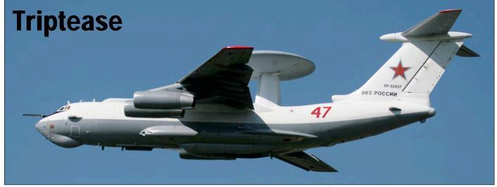
Among the static display highlights of ARMY 2018 at Kubinka air base was this A-50U 47rd/RF-92957. Delivered to the Russian Air Force on 9 December 1986, the Il-76 frame was modified to Beriev A-50U in May 2011. Jan Swart captured the classic engined AEW&C transporter on departure from Kubinka on 27 August 2018.
