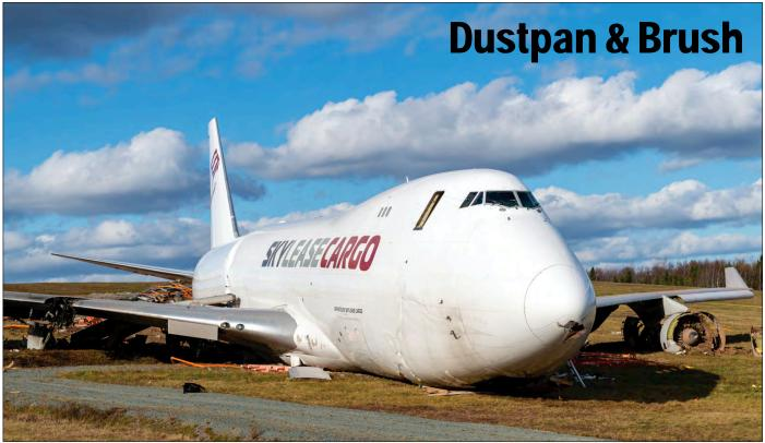
A striking and appropriate opening picture for the Dustpan & Brush! Boeing 747-412F (making this a former Singapore Airlines Cargo aircraft, ex 9V-SFF) N908AR of Sky Lease Cargo was on approach to Halifax-Stanfield International Airport's runway 14, when it overran the runway due to changing wind conditions. You can read part of the transcript between the tower and crew in this section. Marc Geuzinge took this picture on the day of the incident, 7 November 2018.
