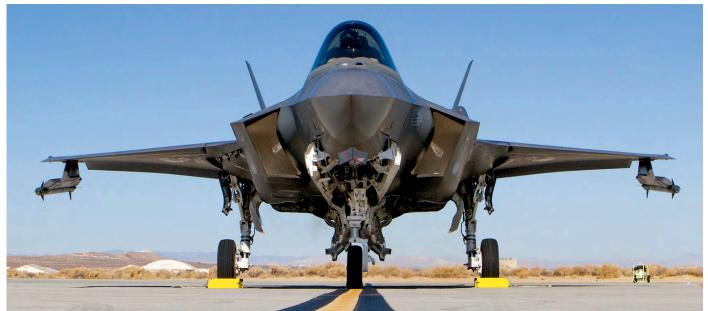
Last summer, some pictures were placed on the Scramble Facebook page of RNLAF F-35A F-001 in Close Air Support (CAS) configuration, the so called "beastmode". In this case, the aircraft is loaded in a much lighter (beastmode light?) configuration with only two Sidewinders as external load. Without doubt this will influence the outstanding Stealth performances of the aircraft negatively. (Arno Gaarthuis)
