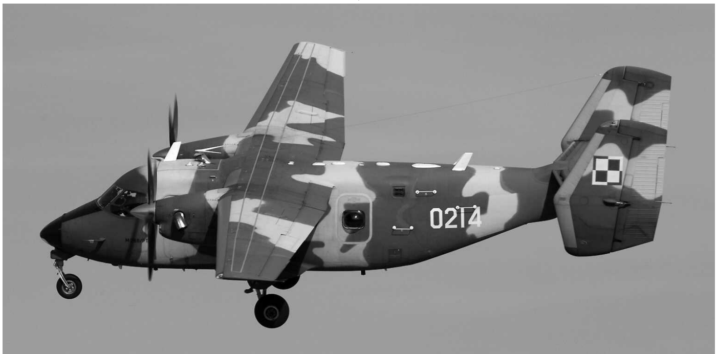
The Polish aviation industry is alive and kicking, producing indigenous aircraft and helicopters. This M-28B/PT is the newest version of the M-28, based on the Antonov 28, but with western engines and avionics. It is now called the Skytruck and also ordered by the USAF Special Operations Command. (Świdwin, 6 October 2009, Piet Luijken)
