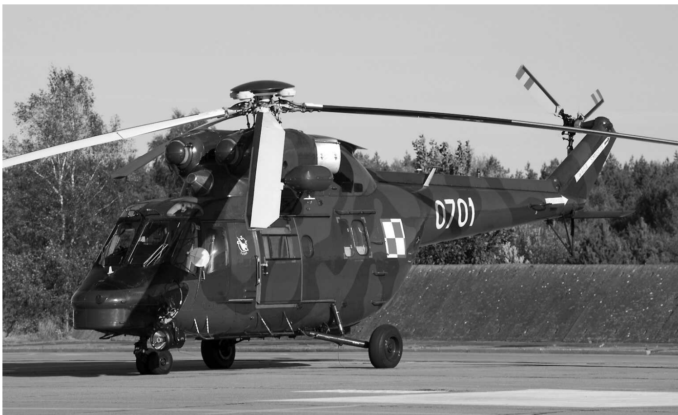
Standing alert in its land rescue/ambulance role, this W-3RL 0701 shows its powerful search light on the left side of its nose and its winch above the sliding door. (Świdwin, 6 October 2009, Piet Luijken)
