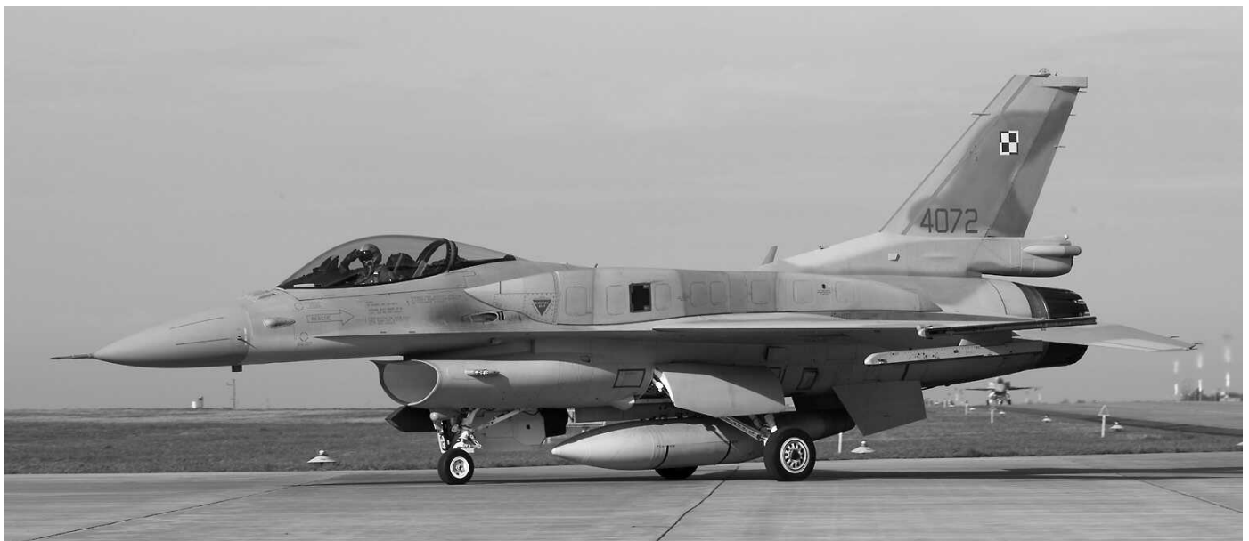
Today, we salute the newest F-16C variant, which can be distinguished by the conformal tanks, shown here by this fine example: 4072 of 10.eltr. The conformal tanks hold 452 gallons each and are carried only on specific air-to-ground missions. Although they give an extra 30 minutes of endurance, extending it into a 2.5 hour range, during air combat they are limited to 8g when fuel is carried or 8.5 g with no fuel in the tanks. This is therefore restricting its purposefulness during pure air policing tasks. Although these conformal tanks can be removed in about two hours, it is policy to have several aircraft dedicated with these tanks.
