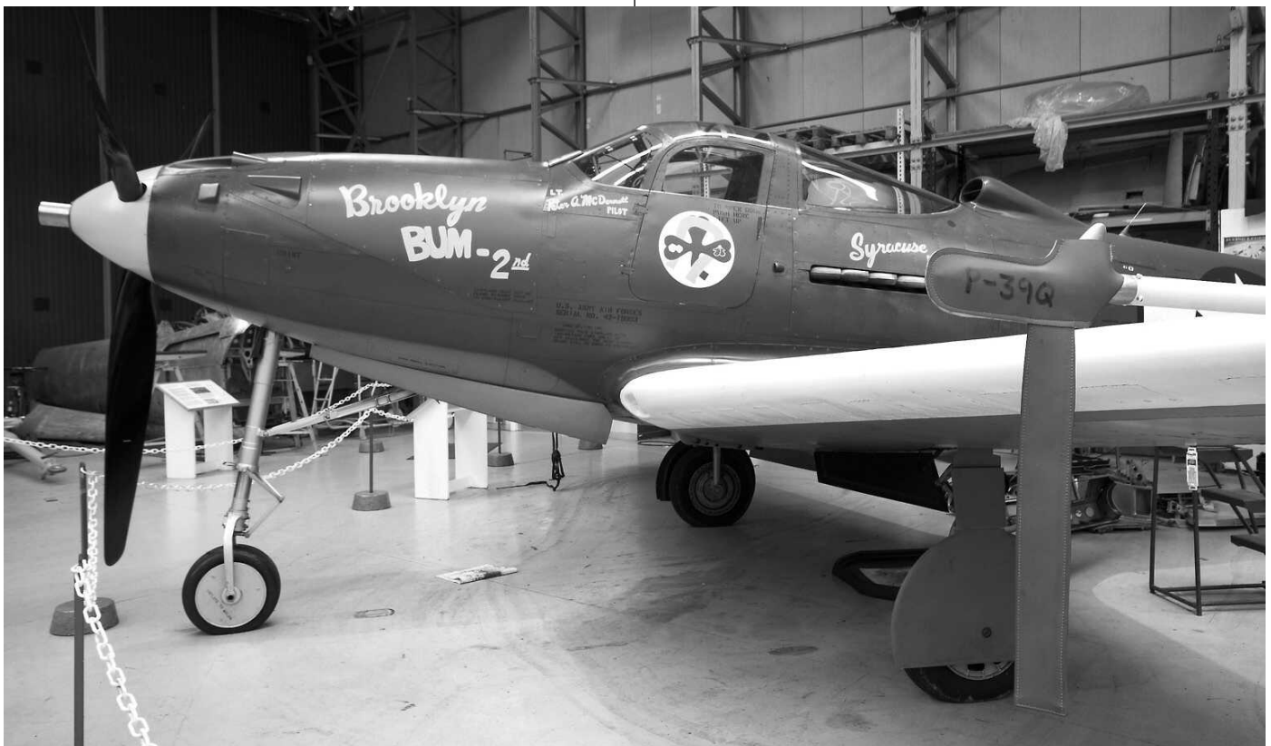
Unfortunately, this Bell P-39Q 42-19993, which was owned and operated by the Fighter Collection at Duxford, has now been sold and shipped to the USA. Its British registration G-CEJU was cancelled by the CAA in January. It seems that the complicated way in which the propellor in this specific aircraft type is driven (through a driveshaft under the cockpit floor) and subsequent technical difficulties played a role in the decision to dispose of the fighter. (Duxford, 13 July 2009, Gert Jan Mentink)
