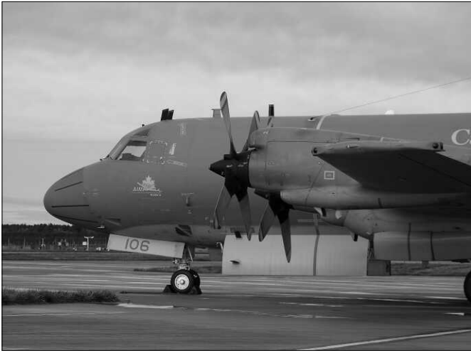
These nose markings identify this Canadian Aurora as an AIMP Block II subtype. In that case, the Aurora Incremental Modernization Program is in the second of four blocks, giving it improved GPS and traffic avoidance systems.
