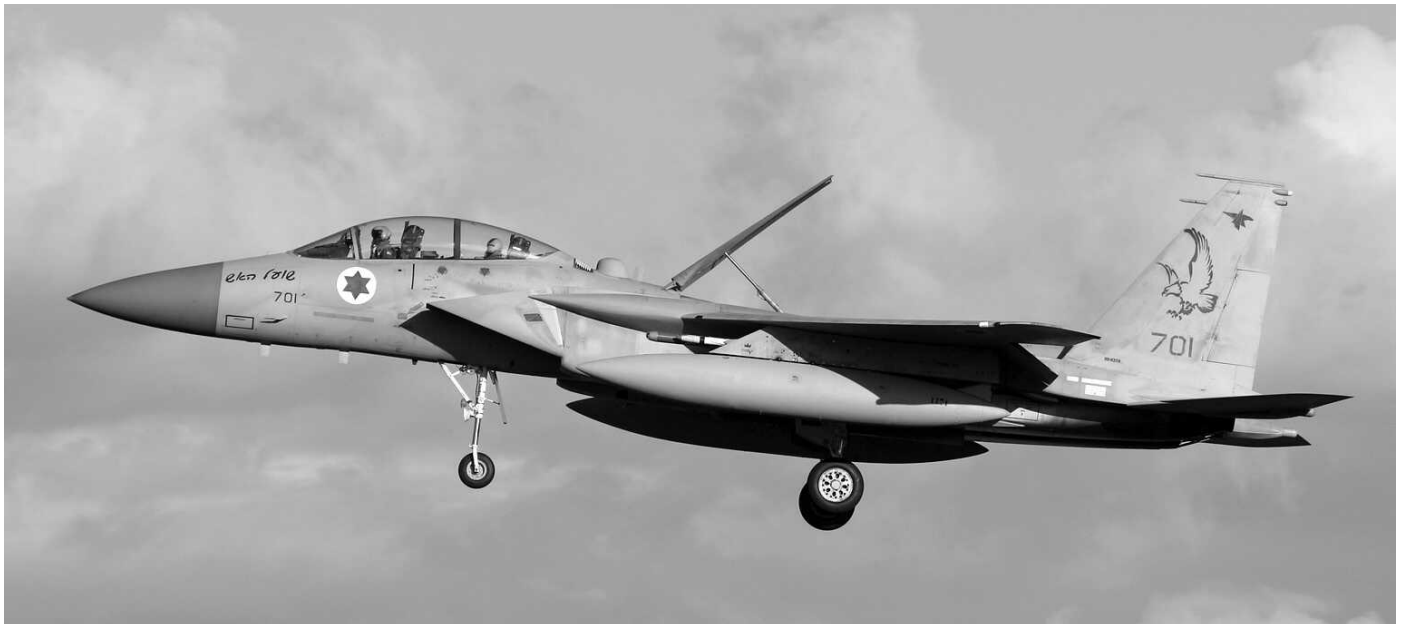
Five F-16s, five F-15s and a single Gulfstream of the IDF/AF took part in the recently held exercise VEGA 2010. F-15D 701 was one of the participants. On the pictures we received, we notice that at least two of the F-15s had a modification behind the canopy. We think this is a satcom device. (Decimomannu, 17 November 2010, Luciano Bertolini)
