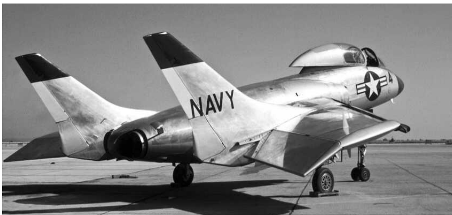
Two shots of 129657/4 on the ramp at NAS Miramar. Note the flightline filled with AD Skyraiders in the background. As can be seen, the Cutlass nosewheel strut had been lengthened to gigantic proportions to improve the airflow over the aircraft's wings, but this size was a contributing factor in the many nose gear failures experienced by the Cutlass.
