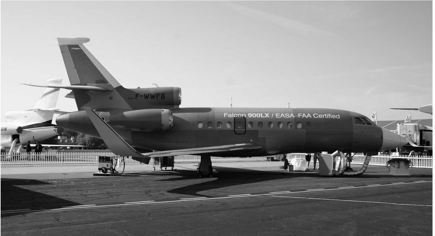
There is still a lot of work that needs to be done before this Falcon 900LX can be delivered to a customer, but Dassault had to show it to the NBAA attendees in support of the FAA and EASA certification of the aircraft. This should not have been too much trouble, as it is basically a Falcon 900EX EASy with winglets. (Edwin Kal)
