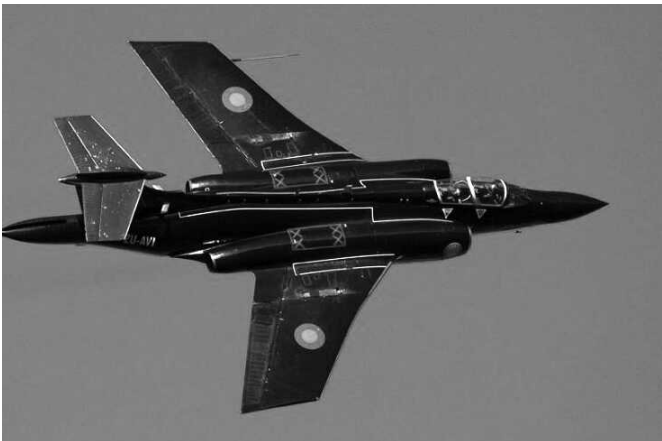
Although the Buccaneer was not a supersonic bomber, it was one of the fastest of its time, able to fly 700 mph at ground level. That is what you call a lawn mower! Here ZU-AVI is seen in a tight turn. (photo Thunder City)
