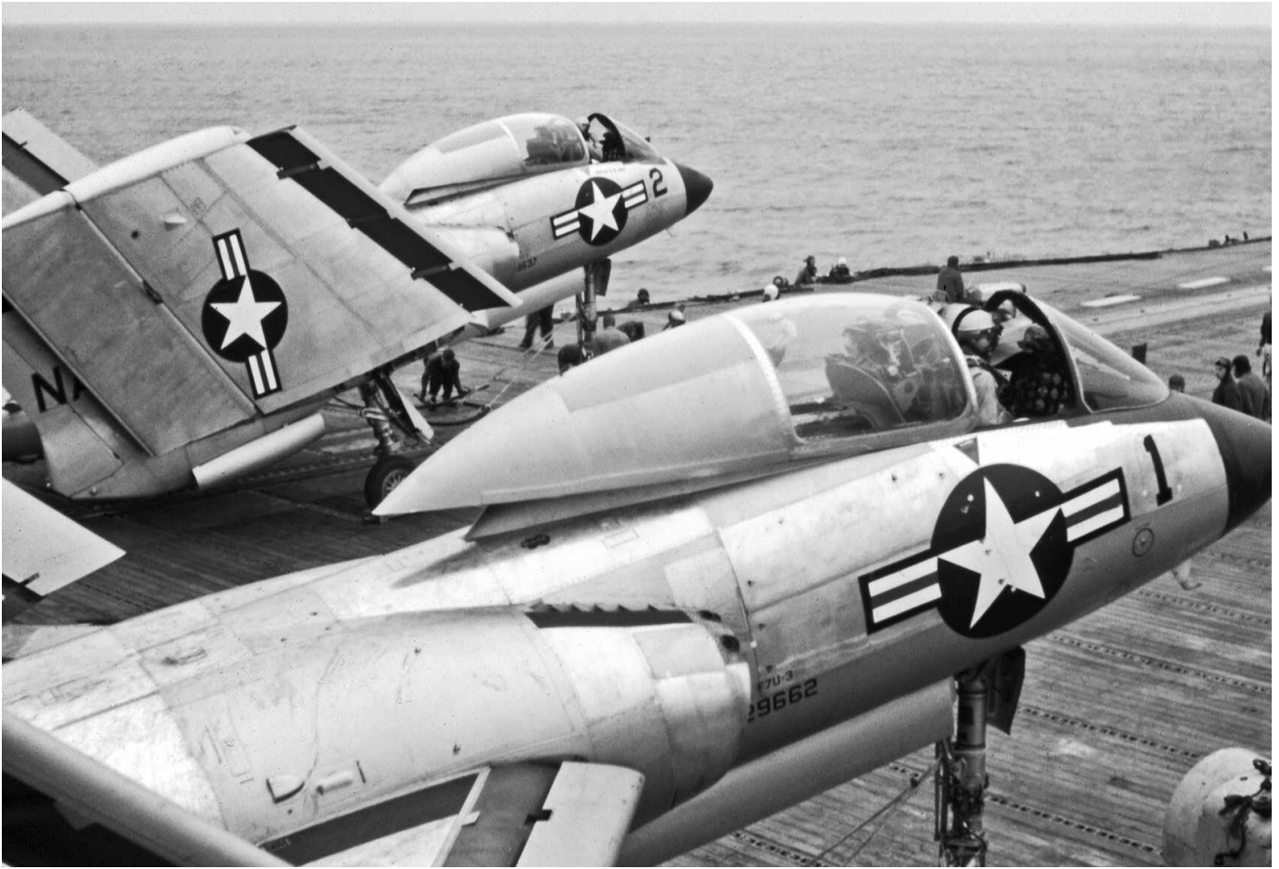
Preparations for the day's flying activities are underway on this photograph taken on board the USS Hancock, with both aircraft being prepared for launch. 129637/2 on top is having its catapult bridle attached. 129662/1 in the foreground offers a nice view inside the cockpit. 'Project Cutlass' markings were very plain, the aircraft had black fin-tips, the legend 'NAVY' was carried on the fin and each aircraft carried an individual code on the forward fuselage, which was repeated on the nosewheel door (see below). The Star & Bar was hi-viz, the area under the wing's leading edge slats was painted red.
