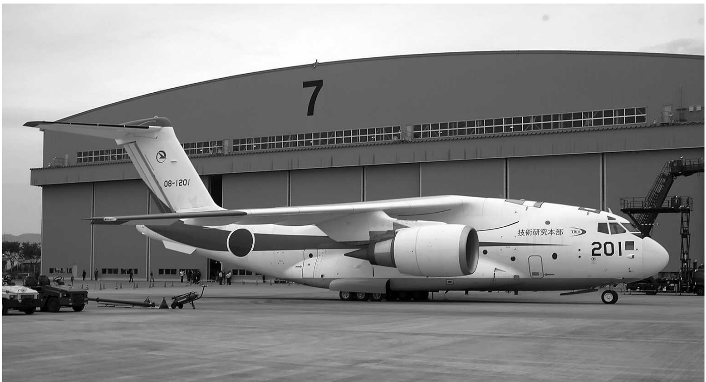
Kawasaki has developed the C-2 as replacement for the C-1 operated by the JASDF. XC-2 08-1201 is the first prototype. (Gifu, 24 October 2010, Frits Jongerman)
