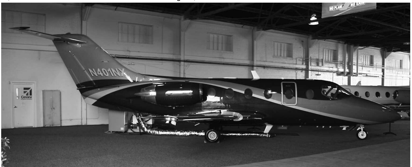
While Hawker Beechcraft introduced a factory retrofit programme for the Hawker 400XP, Nextant Aerospace was actively promoting its upgrade package for the Beech 400 series aircraft, called Beechjet 400XT, but also known as 400XT and previously 400NXT. The main changes are the Rockwell Collins ProLine 21 avionics suite and the Williams FJ44 engines. N401NX is seen here hangared at the static display of the NBAA convention in Atlanta. (Atlanta-DeKalb-Peachtree (GA), October 2010, Edwin Kal)
