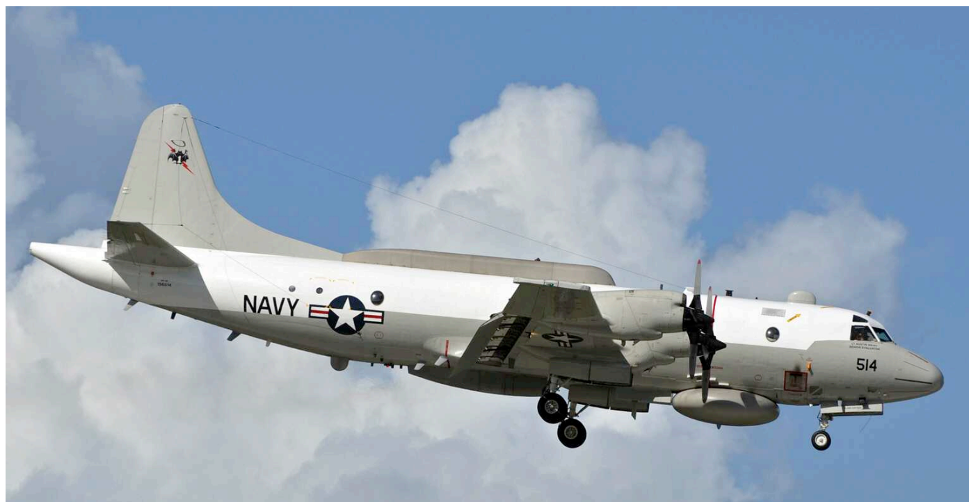
The EP-3E Aries II remains one of the most interesting versions of the Lockheed Orion. This Whidbey Island based VQ-1 Aries II 156514 is used for electronic intelligence gathering from Hato. (13 December 2013, Felix Martina)
