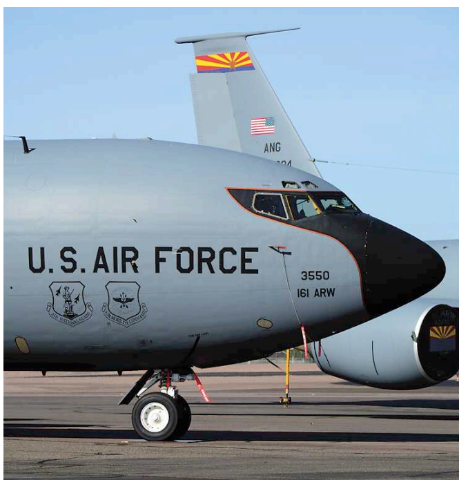
KC-135R 62-3550 has been flying for about seven years with the 197th ARS based at Phoenix Sky Harbor International. This particular aircraft was built in the sixties and is still flying 50 years later! Originally built as KC-135A and later converted to KC-135R. (Phoenix-Sky Harbor (AZ), 8 December 2013, Roy Gorris)
