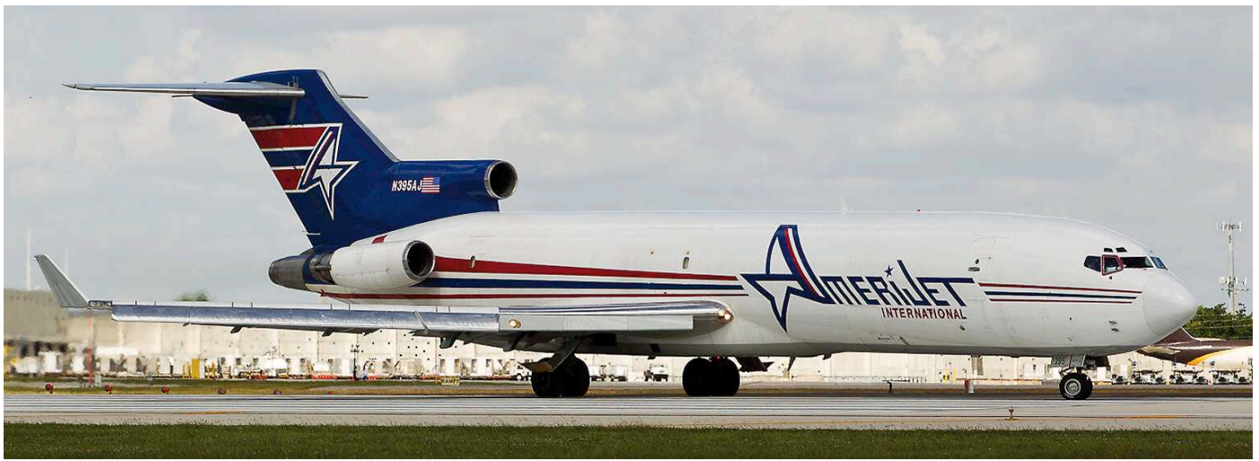
Airfreight International uses N935AJ for ferrying parcels to and from Miami. To comply with regulations, the B727 is equipped with hushkits and winglets for better fuel economy. (Miami-International (FL), 30 October 2013, André Alders)
