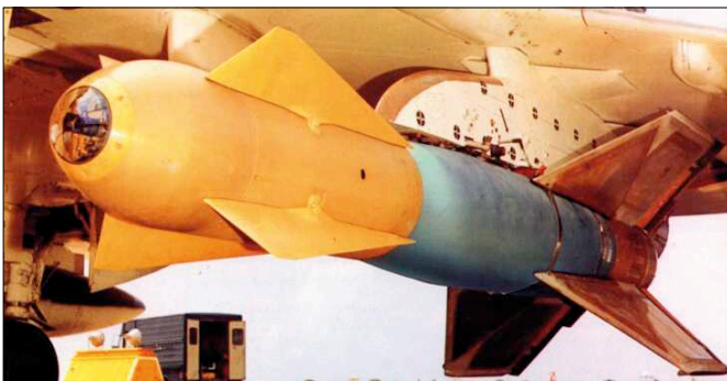
Typical early model GBU-15 Television- or IR Guided Glide Bomb. In the Tunis raid, six of these bombs were used with devastating effect, but one failed to guide properly and probably hit a civilian target.
