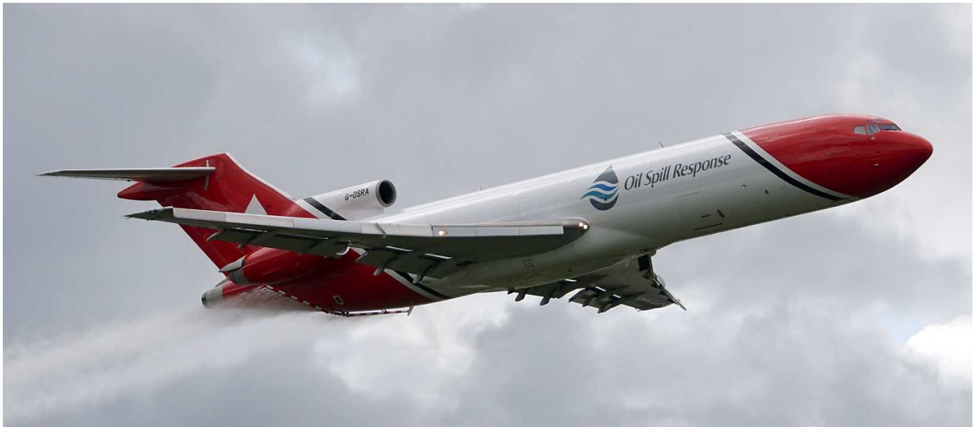
Boeing 727-2S2 G-OSRA is owned by T2 Aviation Ltd. This 727 is operated for Oil Spill Response Limited, together with sister ship G-OSRB. They are both fitted with internal tanks, pumps and a spray boom to deliver dispersant liquid. G-OSRA is seen here demonstrating its capabilities at Farnborough Air Show. (12 July 2016, Lukas Kinneswenger)
