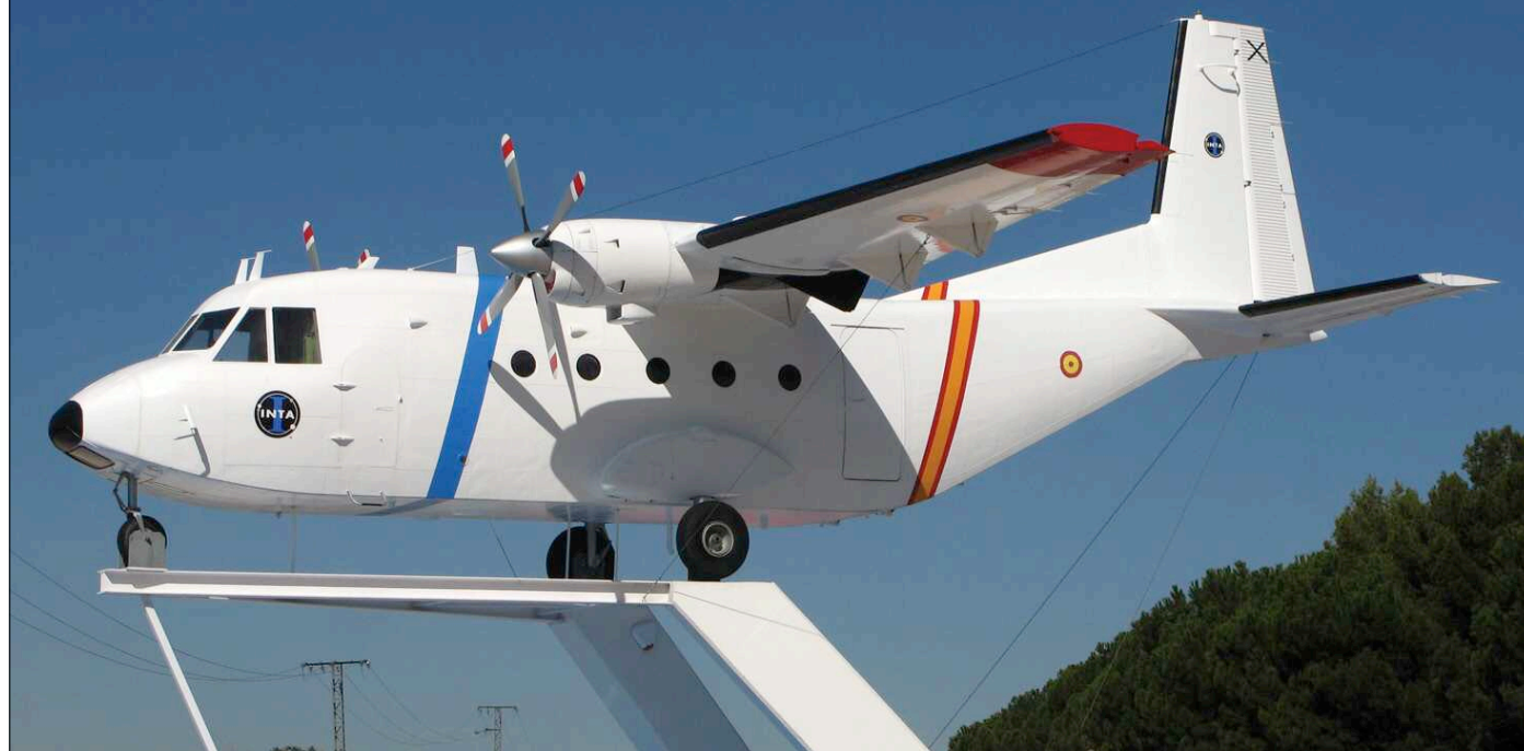
Just outside the INTA gate on the west side of Torrejón is this CASA 212-200 D.3-7. They de-modified the aircraft by removing its large radar nose so it now looks more like a regular INTA CASA. (15 October 2015, Enrique Cortes)
