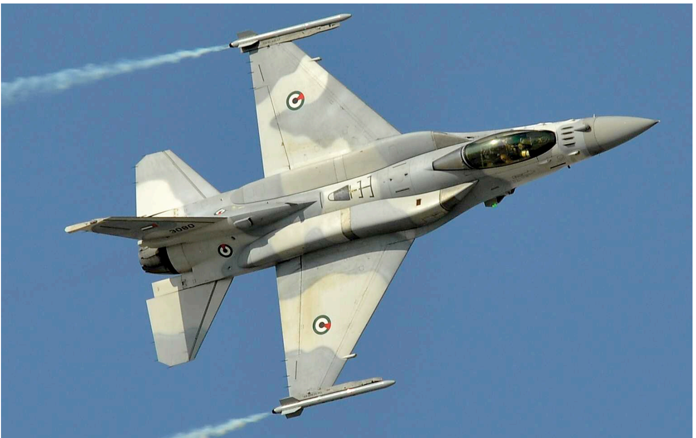
With its conformal fuel tanks much in evidence in this shot, UAE F-16E turns tightly during the Dubai air show at Dubai-World Central. The UAE AF&AD received no less than 82 F-16E/Fs. (F-16E 3080, 7 November 2015, Rene Bremer)
