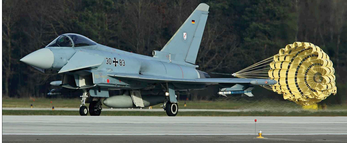
Eurofighter 30+83 of TLG31 is seen here during the roll-out after landing at Manching after a test flight including use of the dragchute. (11 December 2015, Dietmar Fenners)
