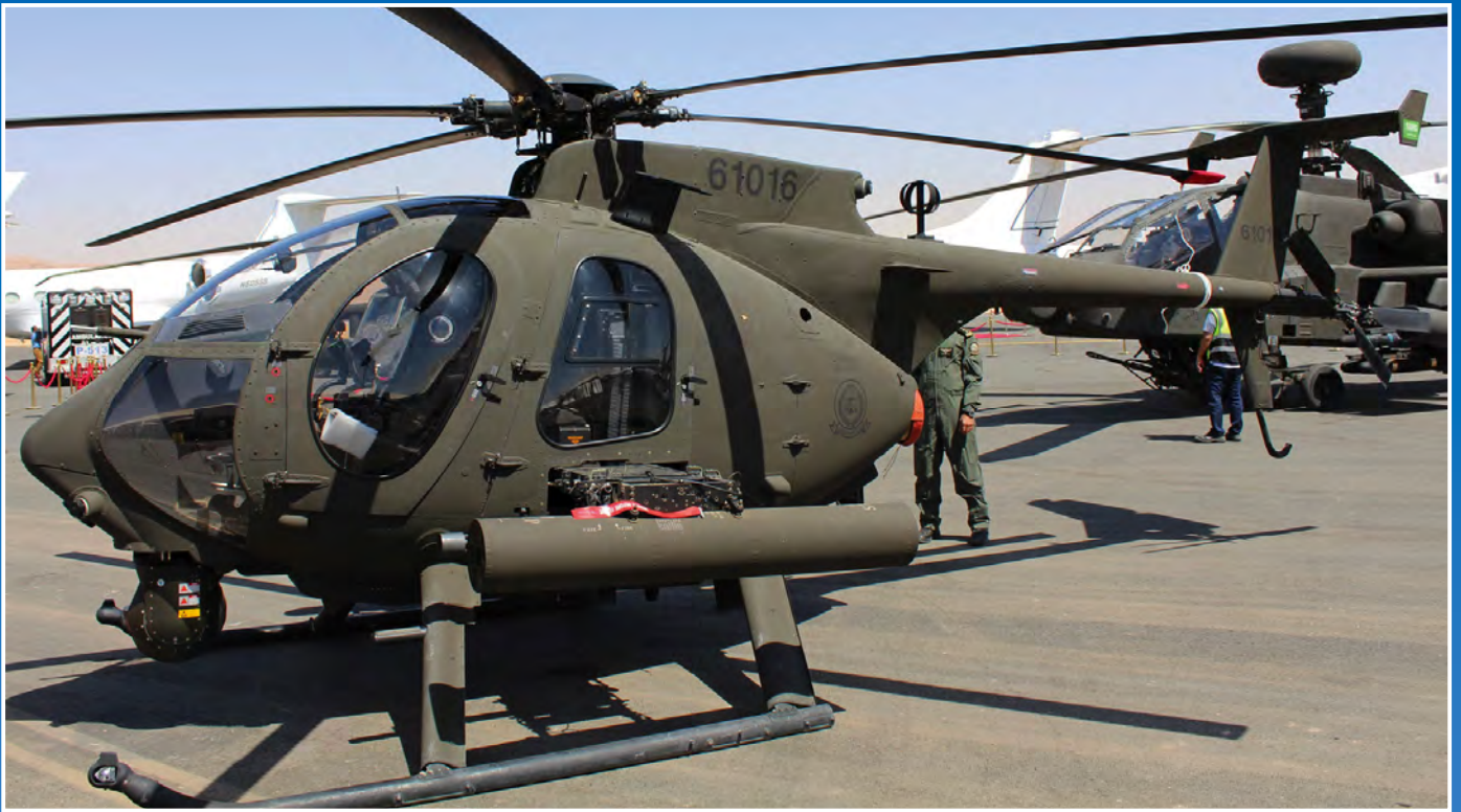
61016 is a Boeing AH-6i and is used by the Saudi Arabia National Guard. Some 36 examples have been ordered and most must have been delivered by now. (Keith Doughty, Al Thumamah, March 2019)
