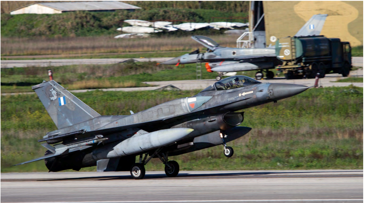
530 is a F-16C block 52+ with Conformal Fuel Tanks (CFT). On the tail is a drawing of a ghost, indicating "Fantasma" 337 Mira is the owner. (24 March 2018)
