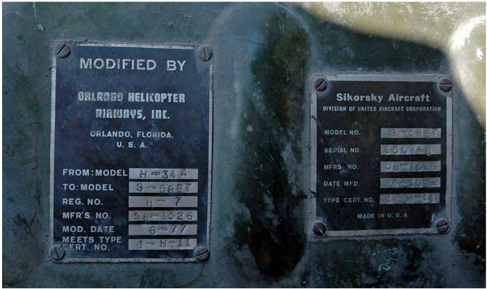
The twin construction number plates of S-58ET H-7 were photographed before the helicopter disappeared from the IDP-camp at the former Bowen Field. To the right is the original Sikorsky plate showing BuNo150748 among other data, and to the left is the plate given by Orlando Helicopter Airways after upgrade to S-58ET, listing Haitian serial number H-7. (03 April 2010, Wim Sonneveld).
