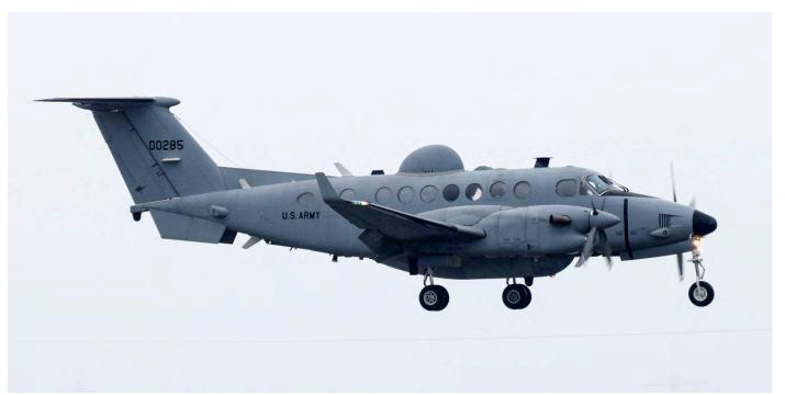
Already operated by the US Army as N8184S since July 2011, this Beech 350i was converted into an MC-12S in 2016 and taken on strength as 11-00285 in December of that year. Most of the aerials and sensors visible in this shot were were already present with its less conspicuous identity, so it is safe to say its Intelligence, Surveillance & Reconnaissance (ISR) role did not start just then. Frank Schuchardt caught the sneaky Beech at a cloudy Wiesbaden on 12 November 2020.
