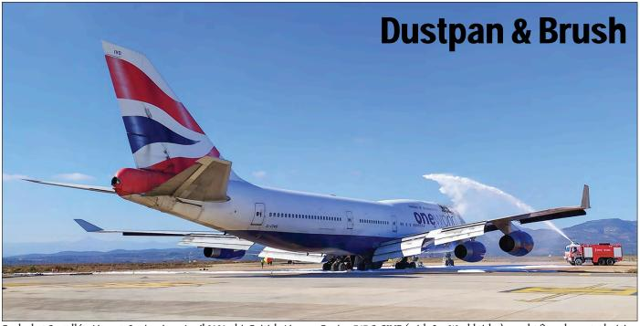
Parked at Castellón Airport, Spain, since April 2020, this British Airways Boeing 747 G-CIVD (with OneWorld titles) caught fire when a technician was cutting an oxygen line on the flight deck and sparks from the cutting wheel were caught by insulation material. Technically, it is not being broken up yet, but given it will be broken up soon, this will go down as a write off. (Castellón Airport Twitter account)
