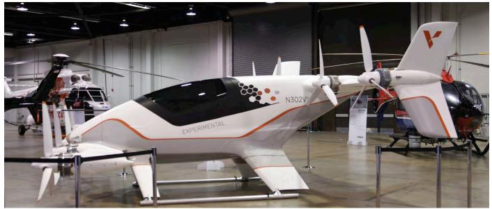
The Vahana is a self-piloted, one seat (unoccupied), eVTOL demonstrator. It has a tested range of 50 km. The configuration is a tandem tilt-wing. This urban-air-mobility concept demonstrator is being retired. The vehicle made its final test flight on 14 November 2019. N302VX made its final appearance at the Heli-Expo. (Anaheim (Ca), 30 January 2020, Kenneth I. Swartz)
