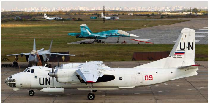
Although Novosibirsk/Tolmachevo is known for its Army Aviation Brigade, it also houses some detachments of other operational Aerospace Forces (VKS Rossia) units. Normally some MiG-31s on QRA can be seen in addition to transport aircraft like this An-30 RF-30080/09(r) of the VKS Rossia which is used for air sampling/radiation reconnaissance. Although in UN colours for over 20 years, it was never used by the UN. (Tolmachevo, 16 September 2019, Andre Alders)
