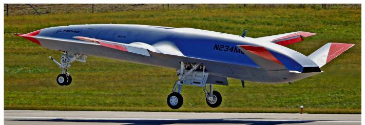
The first flight of the Boeing MQ-25A Stingray Unmanned Aerial System, destined for carrier operations, was on 26 September 2019. It took off from MidAmerica Regional Airport (IL). The UAS completed an autonomous taxi and take-off and then flew a pre-determined route to validate the Stingray's basic flight functions and operations with the ground control station. (Boeing).
