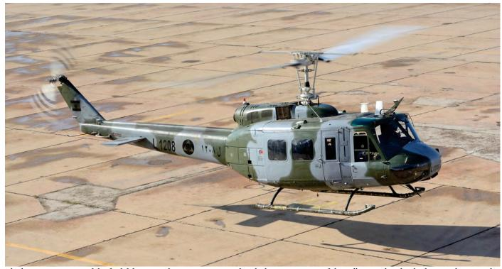
The latest incarnation of the faithful Huey is the Huey II. Equipped with the transmission of the Bell 212 and with a higher rated engine, this has rejuvenated the proven design and they are set to be around for a while yet. After being used in mix with the UH-1H, all Huey IIs are now nominally on 12sq strength; although one was with the Kleyate delegation too.
