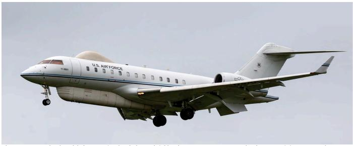
The E-11A is a Bombardier Global Express fitted with the Battlefield Airborne Communications Node. These aircraft function as airborne communication hubs and data links, providing an important translation point between different types of communication. E-11As are often deployed in the Middle East, but are sometimes seen in Europe while transitioning to/from CONUS. (Belfast, 29 July 2018, Paul Harvey)
