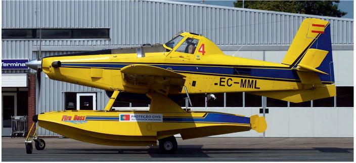
The Fire Boss is an Air Tractor AT-802F equipped with amphibious floats. EC-MML was one of two aircraft stopping for fuel on their way to Sweden, in relation to the forest fires. Judging by the large sticker, this is one of six water bombers operated by Avialsa as subcontractor of the Portuguese company Agro-Montiar. (Goningen - Eelde, 25 July 2018, Hendrik Cazemier)
