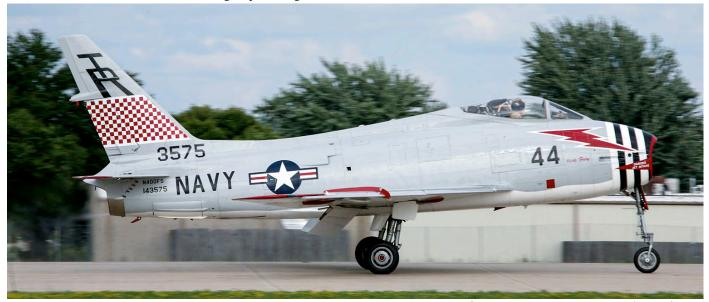
Developed parallel with the more familiar F-86 Sabre, the FJ-4B Fury was a dedicated US Navy/USMC fighter. This Fury, 143575 (N400FS) is the only flying example of its kind. The registration reveals its last operator, Flight Systems, for which it flew from 1977 to 1982 during trials with Pershing missiles. (Oshkosh (WI), 26 July 2018, Ad Jan Altevoqt)
