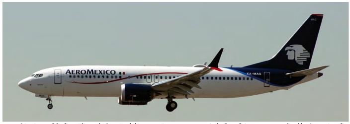
AeroMéxico is one of the first airlines which received the new Boeing 737-8. XA-MAG is the first of nineteen 737-8s ordered by the Mexican flag carrier. It was delivered to Mexico City on 23 February. Besides the typical 737 MAX features (new tail cone design, new ATP winglet and serrated engine cowlings), the AeroMéxico 737-8 MAX aircraft can easily be distinguished from AeroMéxico's 737-800s by their specific XA-MA. registrations. (Mexico City, 31 May 2018, Enrique Giese)
