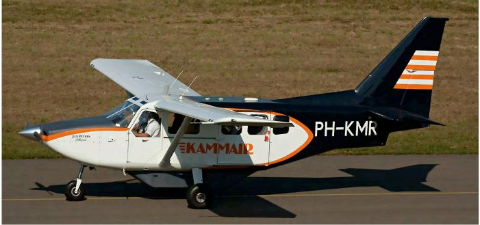
The GippsAero (formerly Gippsland Aeronautics) GA-8 Airvan is a single engine piston utility aircraft developed in Australia. They mainly fly in the outback, just one aircraft is registered in the Netherlands, being PH-KMR shown here. It is similar in appearance to the Explorer 350R on the previous page, but has a fixed gear. (Lelystad, 26 September 2009, Joost de Wit)
