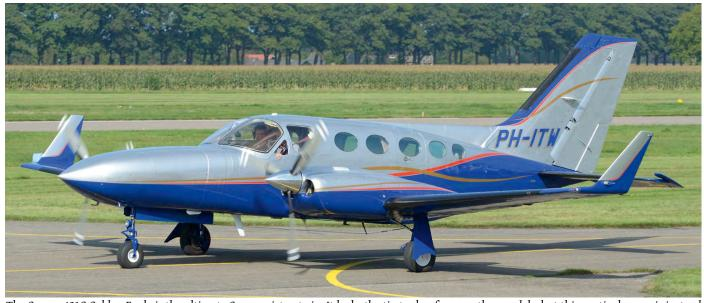
The Cessna 421C Golden Eagle is the ultimate Cessna piston twin. It lacks the tip tanks of many other models, but this particular one is instead equipped with winglets offered by RAM Aircraft, making it a RAM/Cessna 421CW. (Teuge, 12 September 2014, Ron Frijlink)
