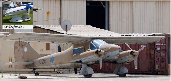
The Dornier 28 is essentially a twin version of the Dornier 27. If you are familiar with that aircraft you will probably recognise the fuselage and wing shape. New are the two piston engines attached to the forward fuselage with struts. Shown here is Do28B-1 026 of the Israeli Air Force. The inset shows the different location of the oil cooler on the Do28A-1. (Sde Dov, 5 May 2008, Erwin van Dijkman)
