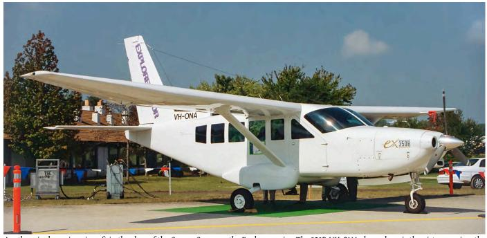
Another single engine aircraft in the class of the Cessna Caravan: the Explorer series. The 350R VH-ONA shown here is the piston version, the turboprop version is called the Explorer 500T. So far production is limited to a few aircraft. Look at the retractable gear to distinguish it from the other high wing single engine aircraft.
