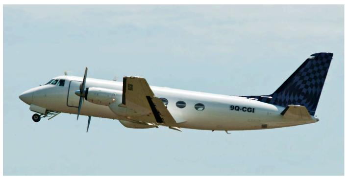
Compared to other bizprops described in this article the Gulfstream I is by far the largest. It is only because it has been developed as a bizprop from the start that it is not categorised as a commuter. The large Gulfstream style cabin windows, as seen on 9Q-CGI, make it standout easily between the commuters. (anonymous)
