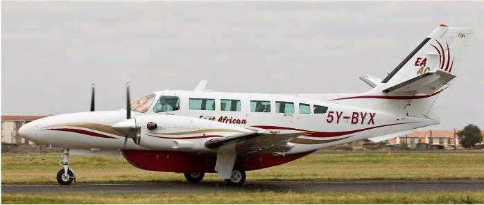
Developed by Cessna, but built by Reims Aviation, is the F406 Caravan II. It has the fuselage and wings of the Cessna 404, but with turboprop engines and a horizontal stabiliser attached to the vertical tailplane. The cargo pod underneath the fuselage shown on 5Y-BYX is optional. (Nairobi-Wilson, 10 August 2014, André Alders)
