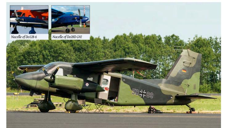
Although the Dornier 28D has a similar arrangement as the earlier variants, it looks more like a different aircraft: it has a much larger fuselage. Most were built as piston version, like this former Luftwaffe Do28D-2 D-ICDY. The small photos show the nacelles of two turboprop versions. (Leeuwarden, 21 June 2008)
