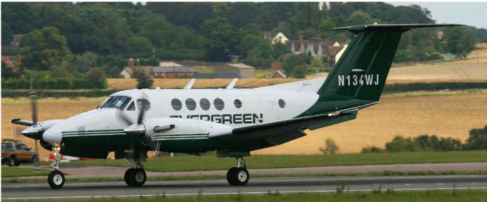
The Beech King Air 200C has a large cargo door on the left hand side. While that is not very clearly visible on this photo, the smaller fifth cabin window is also a recognition point. Also note the original King Air 200 engine nacelles and landing gear doors compared to G-ZVIP above. (Luton, 22 August 2009, John Lythgoe)
