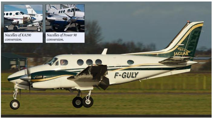
This photo of F-GULY in Jaguar colours shows the general characteristics of the Beechcraft King Air 90 series. It is a King Air C90B, so it has the air intakes extending almost all the way to the prop. Engine upgrades are provided by Smyrna Air Center, as the Power 90 with Walter (GE) engines driving five bladed props. National Flight Service offers the Kilo Alpha 290, with TPE331s, recognised by the large exhaust pipe. (Coningsby, 17 December 2014, Jamie Ewan)
