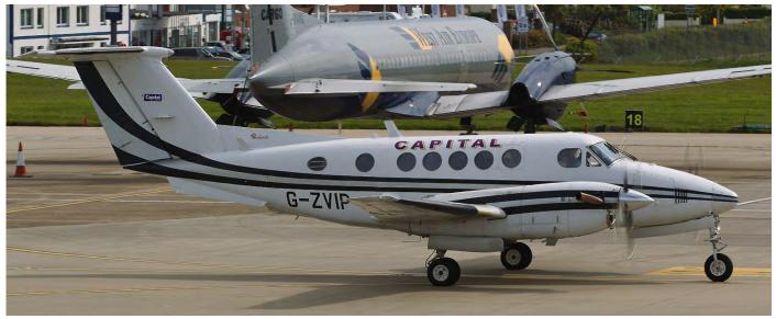
G-ZVIP is a Beech 200 incorporating many upgrades by Raisbeck Engineering: dual aft body strakes, main gear doors fully enclosing the landing gear and baggage lockers at the back of the engine nacelles. (Guernsey, 6 May 2014, André Alders)
