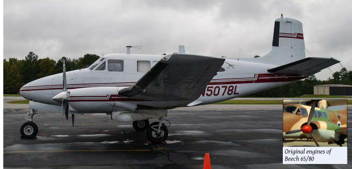
N5078L pictured above was originally built as an L-23F/U-8F for the US Army, which was based on the Beech 65 Queen Air. It has since been converted by Swearingen as the Queen Air 800, as can be seen by the slimmer engine nacelles. For comparison the original nacelles of the Queen Air are shown in the inset. (Griffin (GA), 12 October 2009)
