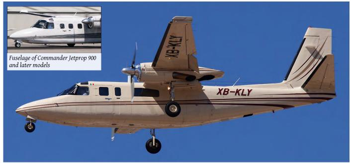
XB-KLY is a Model 690C Commander Jetprop 840, which was the first production model to have (very) small winglets. Furthermore the large panorama cabin window is clearly visible on this approach shot by Joris Termorshuizen. The detail on the left shows the larger number of square windows instead of the panorama window. (Tucson (AZ), 11 April 2012)
