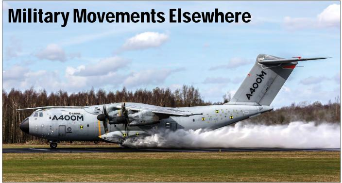
Only days before the dormant Twente Air Base was turned over to civilian control Airbus had contracted Dutch NLR for a couple of standing water runway tests. Prototype A400M EC-402 was used for the trials. (Twente, 21 March 2017, Pascal van Uffelen)
