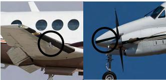
You can tell if the King Air 90 is an early model (90, A90, B90 or C90) by looking at the location of pitot tube: it is underneath the wing (left photo). Later models have it on each side of the nose.
