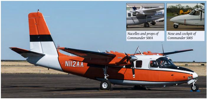
The second generation of piston-powered Commanders has slimmer engine nacelles, clearly visible on N112AA, a Commander 500B. The main gear rotates ninety degrees before it is stored in the back of the nacelles. The Commander 500A has two-bladed props as can be seen in the first detail photo. The last short-body Commanders (500Ss and most 500Us) have a pointier nose and different cockpit windows, including a so-called 'eyebrow' window. (Denver-Front Range Airport (CO), 2 October 2012)
