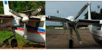
These two details show the difference between the early model Turbo Commanders and the later models, from 690 on. On the Commander 690 the engines are further from the fuselage, so that larger propellers can be used. As you can see the difference in prop diameter is significant.
