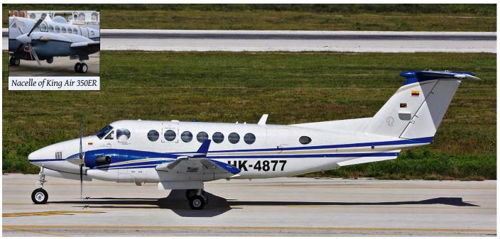
You count seven cabin windows on this King Air (forgetting about the one right of the cabin door), which makes it a King Air 350. It has no large cargo door, so it is no King Air 350C. And while the aircraft has extended engine nacelles (modified by Raisbeck), it is no King Air 350ER either. The nacelles of that version are even larger (see small photo). (Curaçao-Hato, 21 December 2012, Larry Every)
