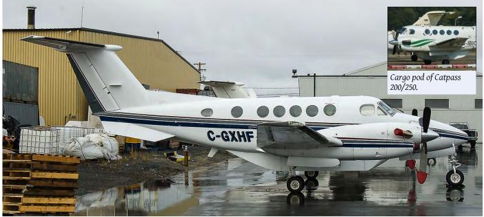
Beechcraft developed a high-density version of the Super King Air for the commuter market. It was traded as the Beech 1300. The large cargo pod underneath the fuselage used for the baggage is clearly visible on C-GXHF above. The small photo shows the somewhat smaller cargo pod of the Catpass conversion offered by Commuter Air Technology. (Yellowknife (N.W.T.), 15 September 2008)
