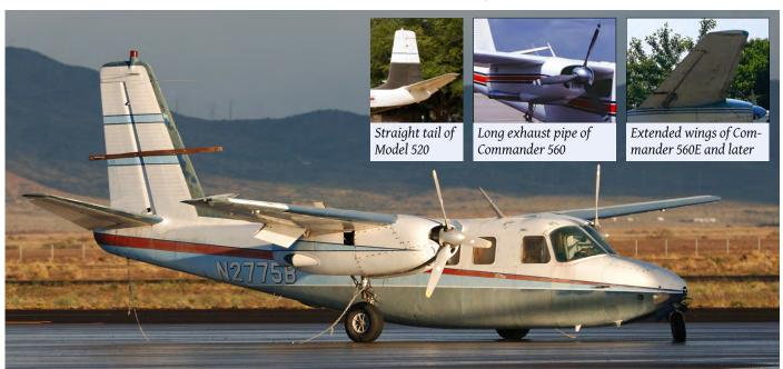
This photo of Commander 560A N2775B shows the characteristics of the first generation of Aero Commanders. These are recognisable by the "bulky" engine nacelles. Model 560A has a swept vertical tail, unlike that of Model 520 (see first inset). Both Commander 520 and 560 have a long external exhaust pipe; the visible part of the Commander 560A is much smaller. (Kingman (AZ), 22 November 2010, Ron Frijlink)
