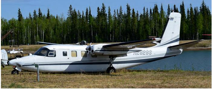
The model 680FL Grand Commander was the first stretched version. It normally has four cabin windows on each side, although there are known conversions with the panoramic window of the 690. Then it can still be recognised by the old blunt nose (don't be fooled by the radar nose) and the somewhat rounded vertical tail. These two characteristics also differentiate models 680T and 680V from the 680W, 681 and 690 series. (Fairbanks (AK), 14 May 2015, Walter Heukensfeld)
