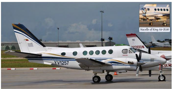
The Beech 100 is a stretched version of the Beech 90, which thus has more cabin windows. Also it has two wheels on each main landing gear. YV1257 is a Beech A100 and has four bladed props as a standard. In addition this particular aircraft has redesigned engine intakes, which more resemble those of the King Air C90A. The inset shows the nacelle of the King Air B100. Note the large exhaust pipe! (Aruba, 22 October 2010, Ruud Fopma)
