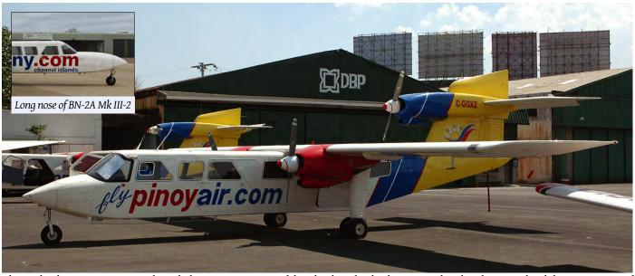
The Trislander is in essence an enlarged, three engine version of the Islander. The third engine is placed in the vertical stabiliser. C-GOXZ is of the first variant, the BN-2A Mk III-1. The inset shows the longer nose of later versions. (Manila, 9 March 2010, Ron Mak)
